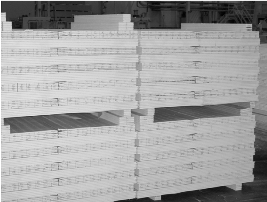
Figure 1 – Typical Gypsum Risers
